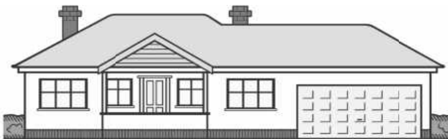
The general pattern of new residences is to have garages incorporated under the main house roof. This damages traditional proportions and is not accepted practice in heritage design.
