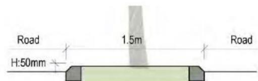
Detail for median - enable tree planting whilst allowing for vehicle movement and providing pedestrian refuge.
