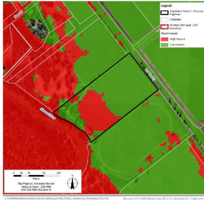
Figure 10-8 Candidate Area 2 – Flood Hazard
