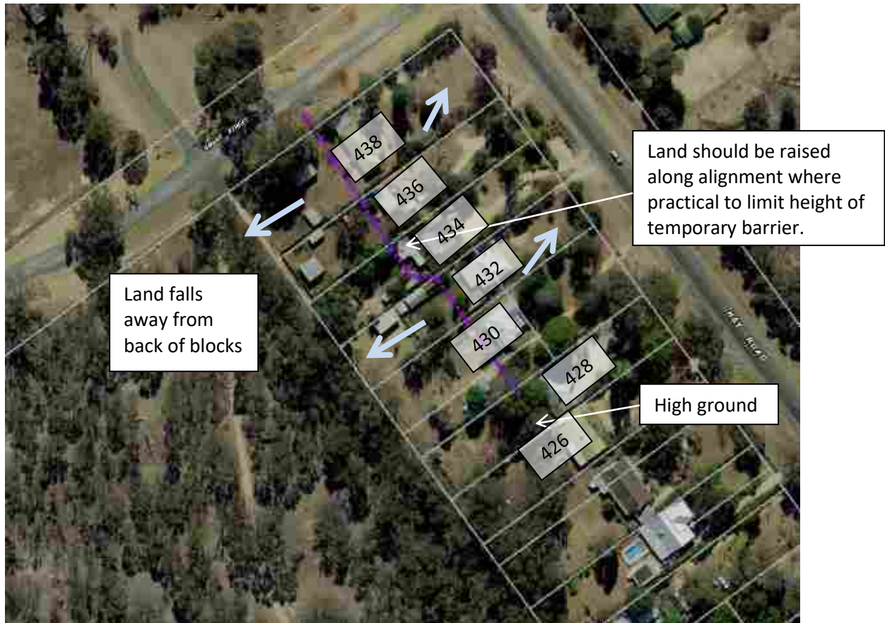
Figure 25: Section 9 - Temporary Levee through properties No. 438 to 428 Hay rd.
