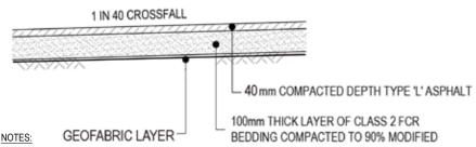
'D' = DEPTH OF ASPHALT FOOTPATH
