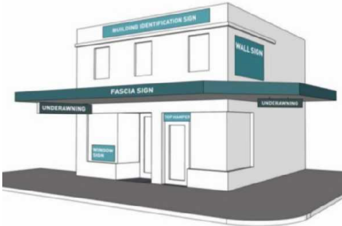
Figure 13-1 Types of Signs (Source: NSW Planning and Infrastructure, Changes to Exempt and Complying Development - Information Sessions for Council and Industry Practitioners January 2014 – February 2014)
