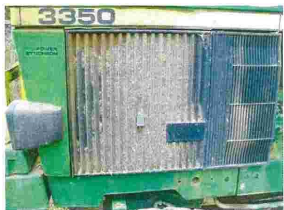
Tractor driven slasher – radiator loaded with weed seeds
